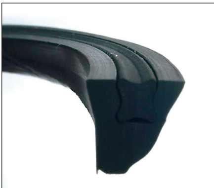
Fig. 2-7. Instability failure of a square profile piston seal
